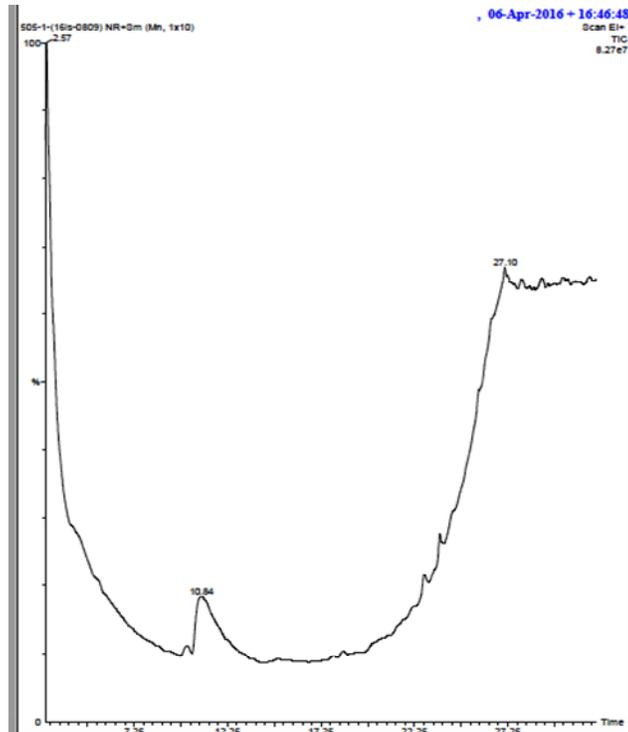
**Figure7.** GC-MS Peaks with Retention Time (RT) for degraded metabolite by the bacterial consortium
