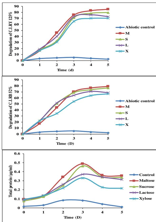
**Figure 10.** Effect of carbon sources on decolorization of mixed reactive dyes (C.I.RY 125 and C.I.RB 52) and total protein content (100 ppm).
