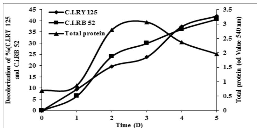
**Figure 15.** Decolorization of mixed reactive azo dyes (C.I.RY 125 and C.I.RB 52) in the treatment of textile effluent
