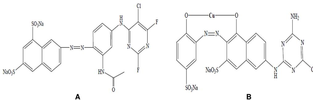
**Figure 1.** Shows the Structure of the reactive azo dyes (A) C.I. Reactive Yellow 125, (B) C.I. Reactive Blue 52
