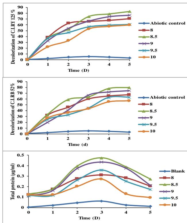
**Figure 8.** Effect of pH on decolorization of Mixed reactive azo dyes C.I.RY 125 and C.I.RB 52 Dye and total protein content (100 ppm)
