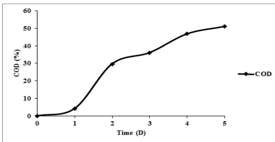
**Figure 16.** Removal of COD from the synthetic textile effluent wastewater
