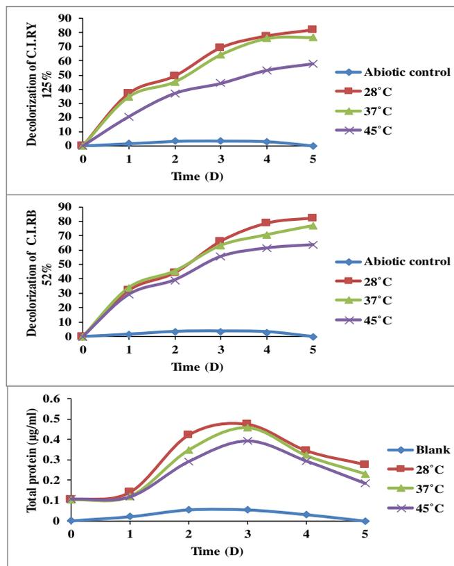
**Figure 9.** Decolorization of mixed Reactive azo dyes (C.I.RY 125 and C.I.RB 52) at different temperature by the isolated bacterial consortium
