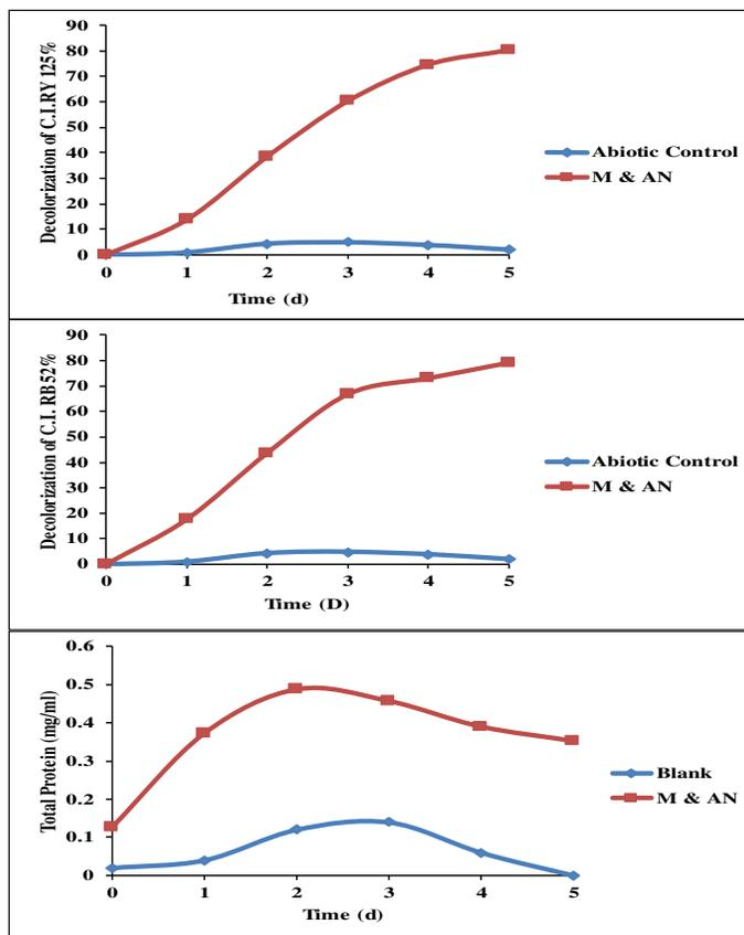
**Figure 12.** Effect of Mixed carbon and nitrogen sources on decolorization of mixed reactive azo dyes (C.I.RY 125 and C.I.RB 52) and total protein content
