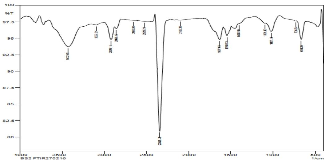
**Figure 5.** FTIR Spectrum of Mixed Reactive Azo dyes (C.I.RY 125 and C.I.RB 52)
