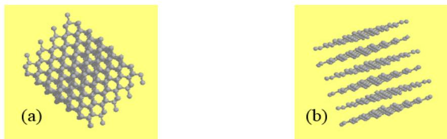
**Figure 1.** (a) Diamond structure and (b) graphite's layered structure (Ozaki et al., 1998).
